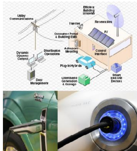
Figure 3. V2G system design [9]
