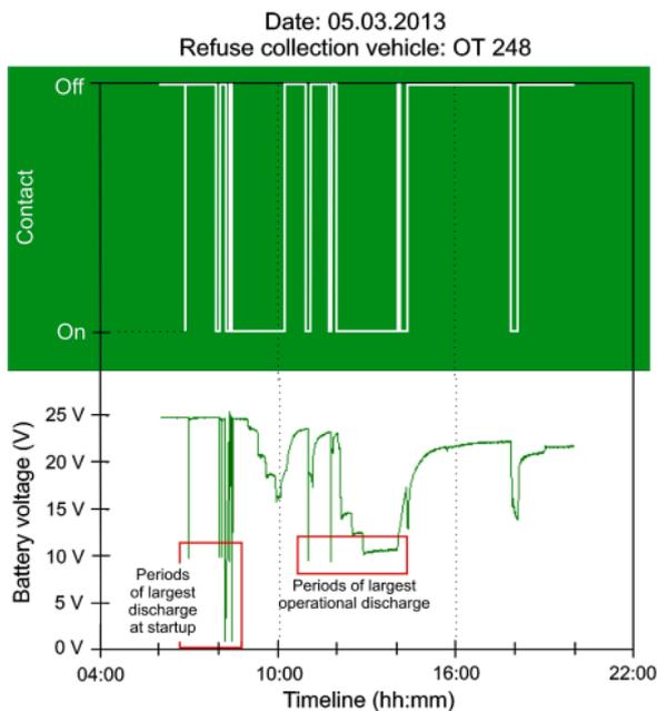
Figure 4. A problem of continuous battery discharge
