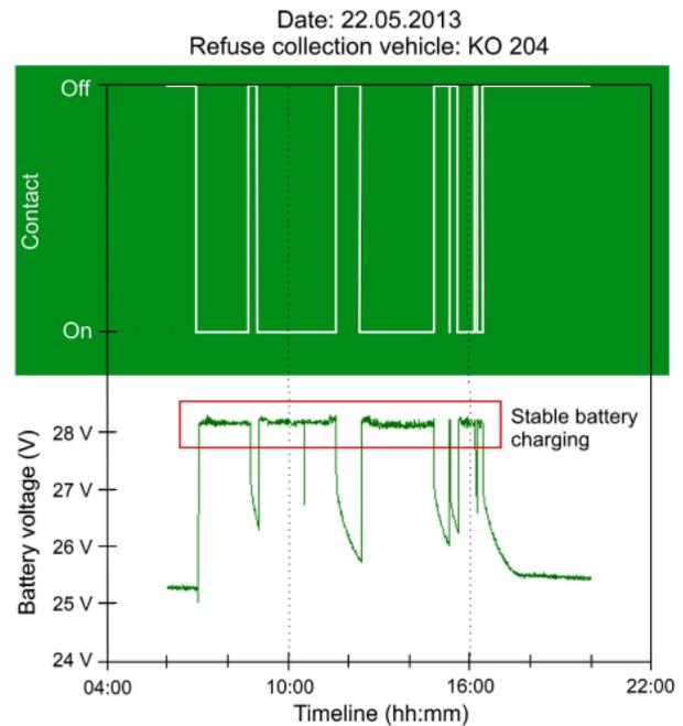
Figure 5. An example of good battery charging system
