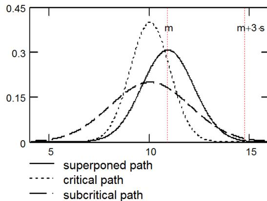
Figure 3. The distributions of probability of the critical, subcritical and superponed time flow
