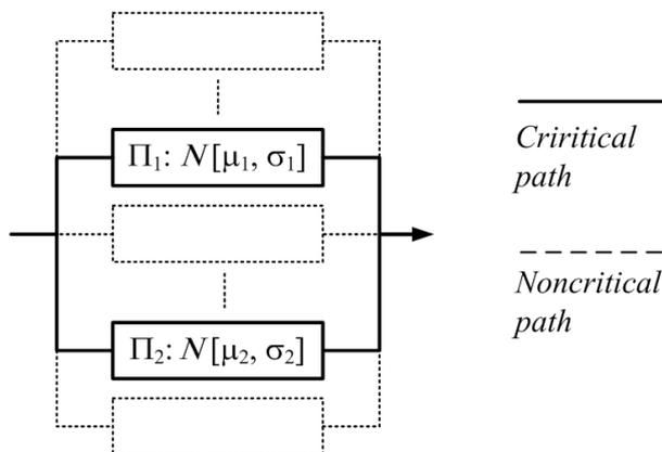
**Figure 1. The flow network with the two locally - autonomous critical flows of PDM structure activity**
