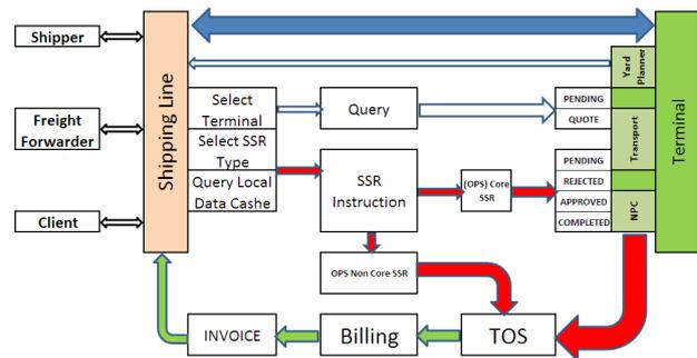
Figure 3. SSR workflow diagram
