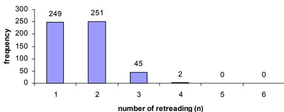
Figure 6b. Empirical distribution density of total number of retreading (till writing-off) on analysed sample of tires „Kormoran“
