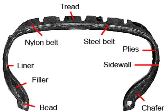
Figure 3. Typical structure of tire (cross section)
