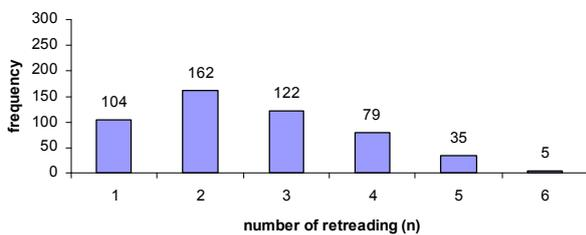
Figure 6a. Empirical distribution density of total number of retreading (till writing-off) on analysed sample of tires „Sava“
