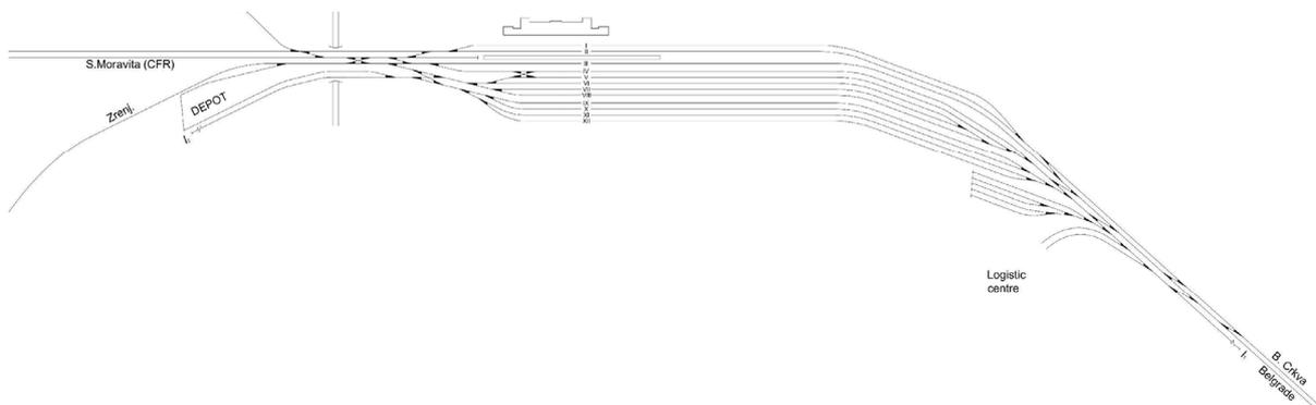
Figure 3. The reconstructed layout of Vršac railway yard
