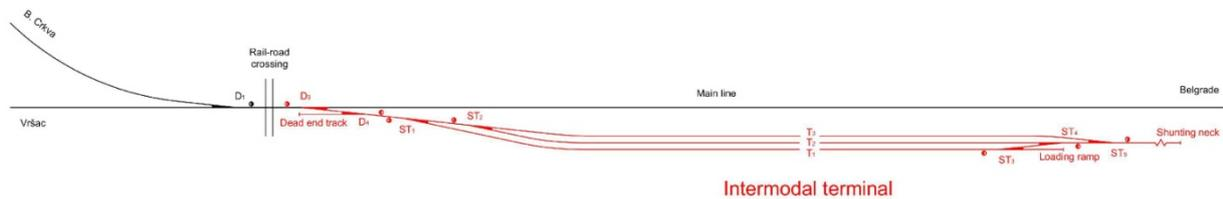
Figure 4. The layout of the rail-road transshipment yard
