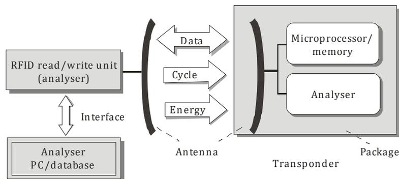
Figure 1. Functioning principle of an RFID system (VDI 4472, 2006)
