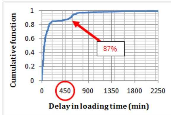
Figure 2. Cumulative function of measured out delays
